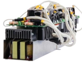
View of the PBI rectifier power block
