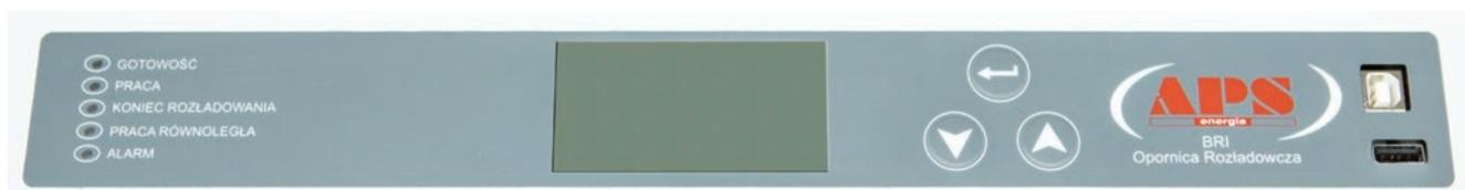
The controlled discharge process parameters are set via 3-button keyboard and the graphic LCD located on the front panel or remotely through RS485 or USB links. Discharge is carried out until the battery's voltage reaches the set minimum level or until the set discharge time elapses.
