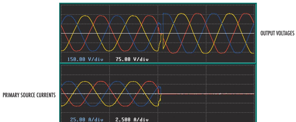
Fig. 15. SSTN transfer to redundant power source initiated by power interruption on preferred input source.
