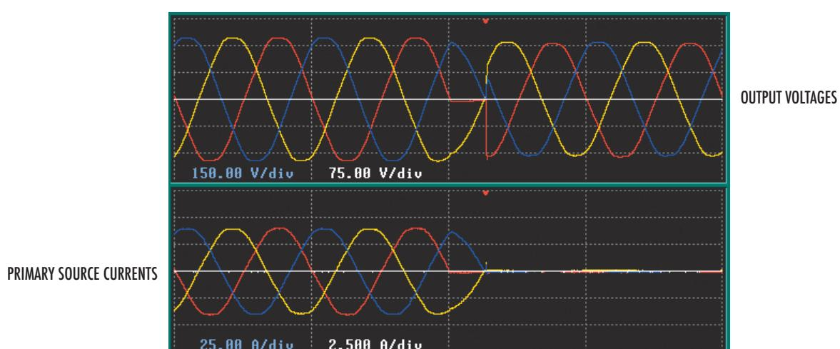
Fig. 14. SSTN transfer to redundant power source caused by power swell on preferred input source.
