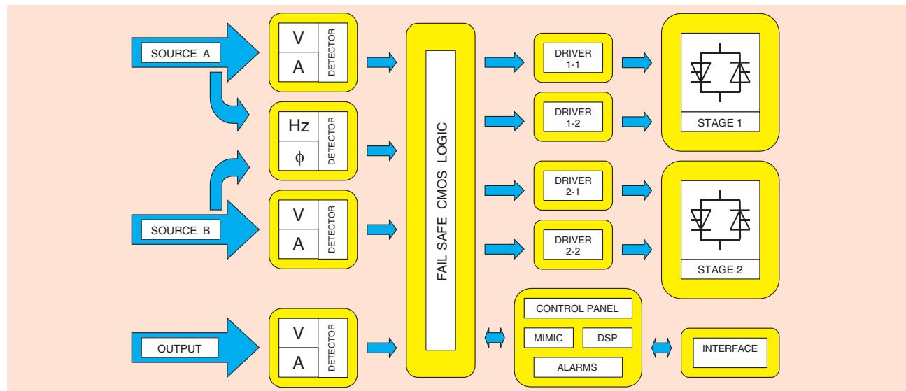
Fig. 2. Block diagram of STS control unit.
