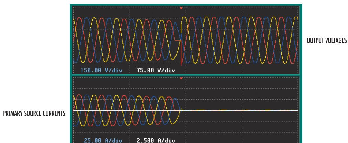
Fig. 13. SSTN transfer to redundant power source caused by power sag on preferred input source.
