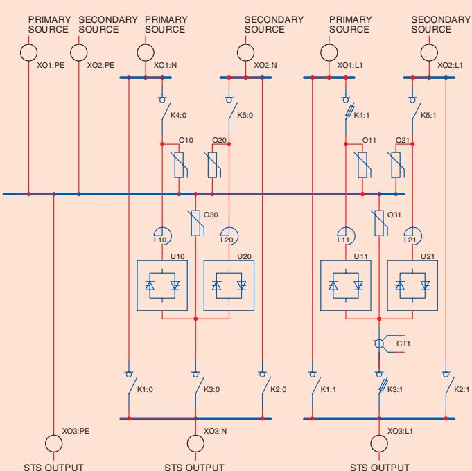
Fig. 5. Power stage circuit of 1-phase 2-poles switch SSN.
