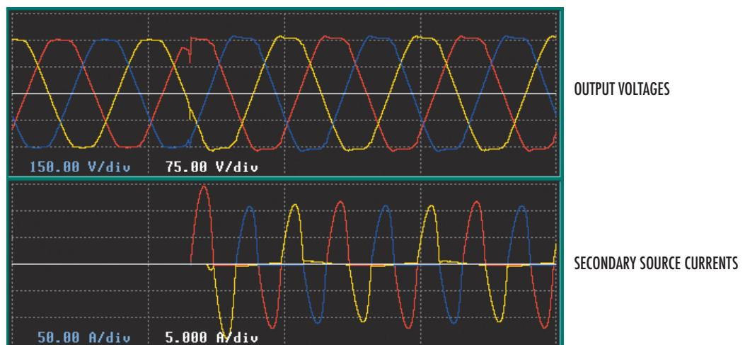
Fig. 17. SSTN transfer to redundant synchronised power source – computer load.
