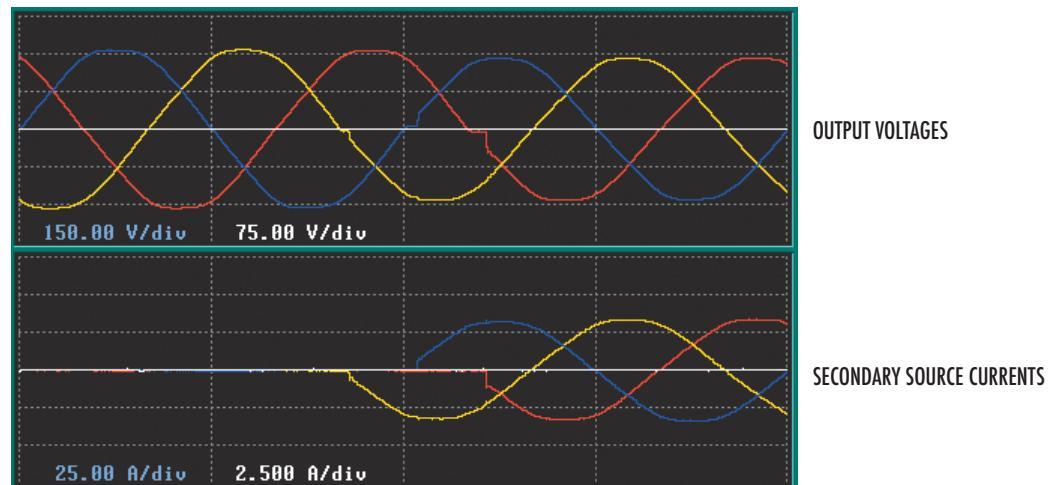
Fig. 12. SST transfer to redundant power source initiated by change of preferred input source.
