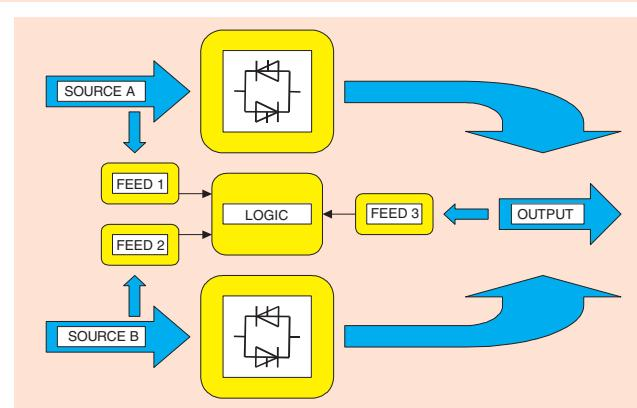
Fig. 3. Internal supply redundancy system concept.
