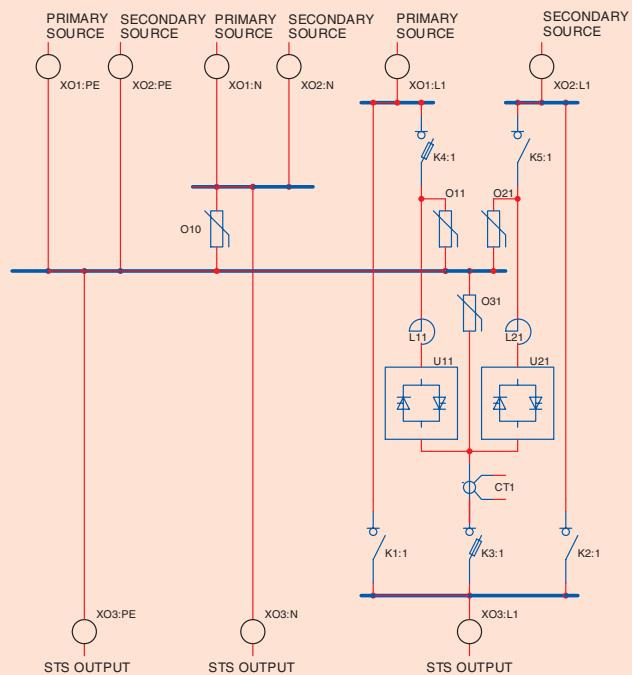
Fig. 4. Power stage circuit of 1-phase 1-pole switch SS.
