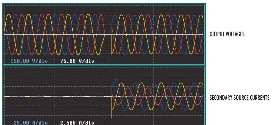
Fig. 16. SSTN transfer to redundant unsynchronised power source initiated by change of preferred input source – asymmetrical load.
