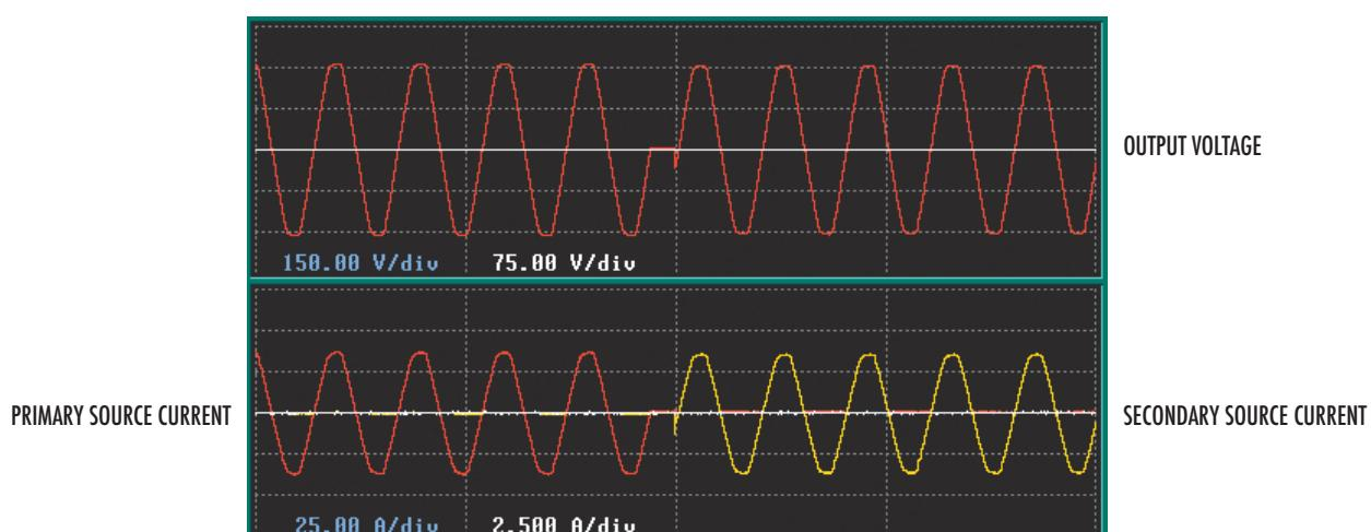
Fig. 11. SS transfer to redundant power source – unsynchronised lines.
