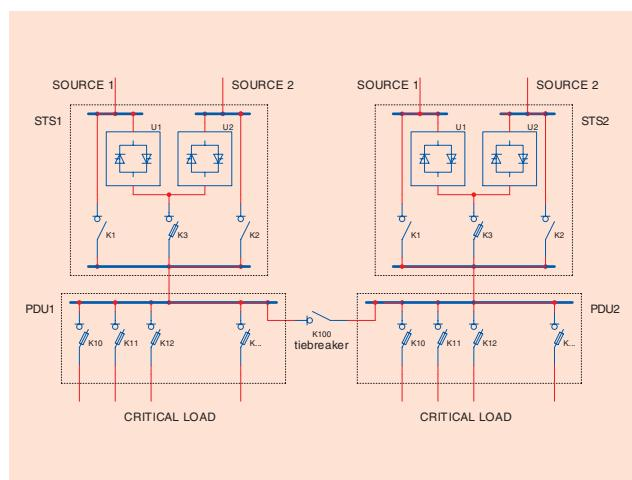
Fig. 19. Two-STS set for two-section power distribution unit with tiebreaker.
