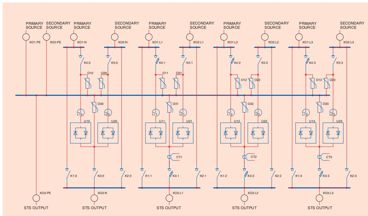
Fig. 7. Power stage circuit of 3-phases 4-poles switch SSTN.
