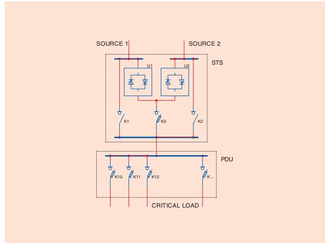
Fig. 18. STS set for power distribution unit.
