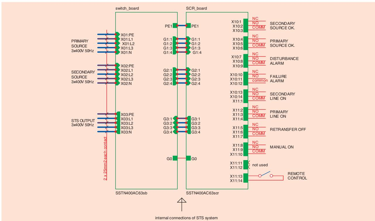
Fig. 8. An example of a SSTN400AC63 rack installation diagram. NC - Normally close, NO - Normally open.
