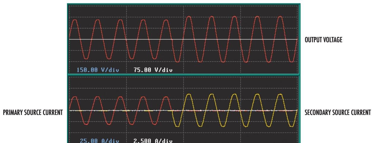
Fig. 9. SS transfer to redundant power source initiated by change of preferred input source.
