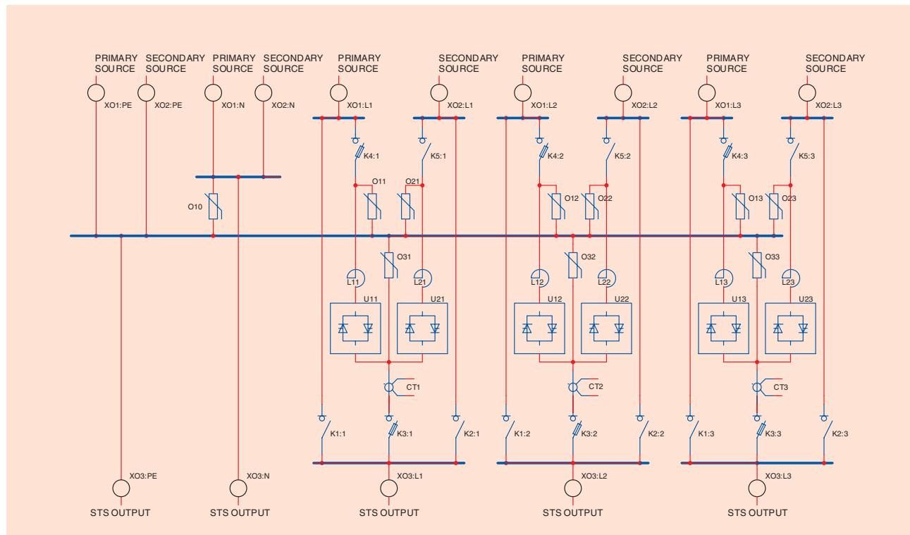
Fig. 6. Power stage circuit of 3-phases 3-poles switch SST.
