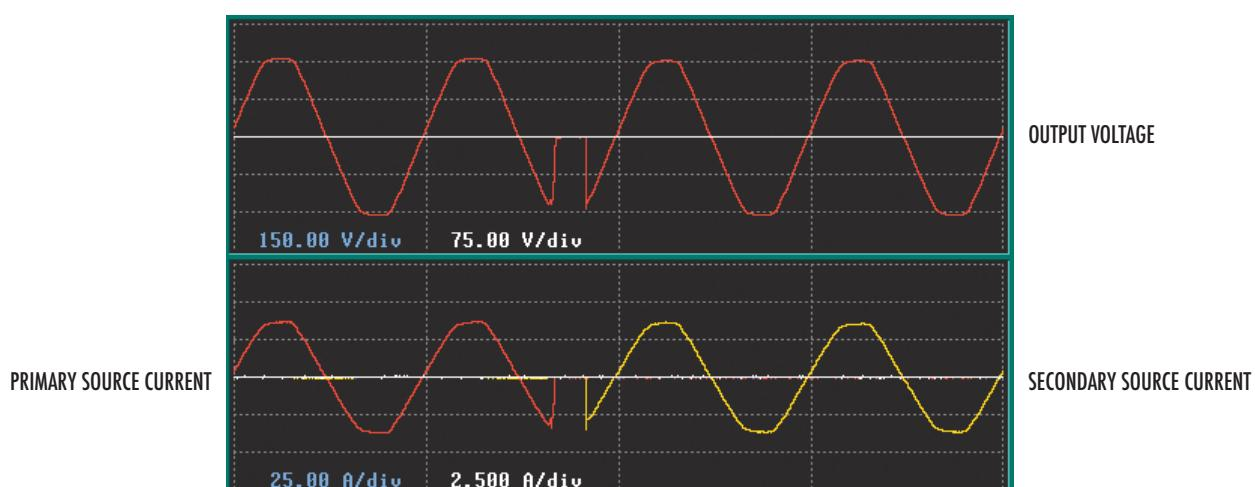
Fig. 10. SS transfer to redundant power source caused by power interruption on preferred input source.
