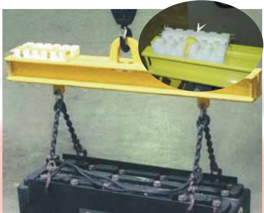
Proper hook position for battery size and correct hook angle
